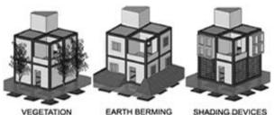
Figure 8: Multiple ways to avoid heat gain due to solar radiation
