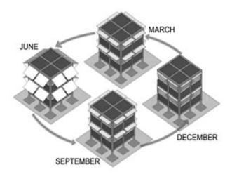
Figure 6: Positions of operable shading devices year round
